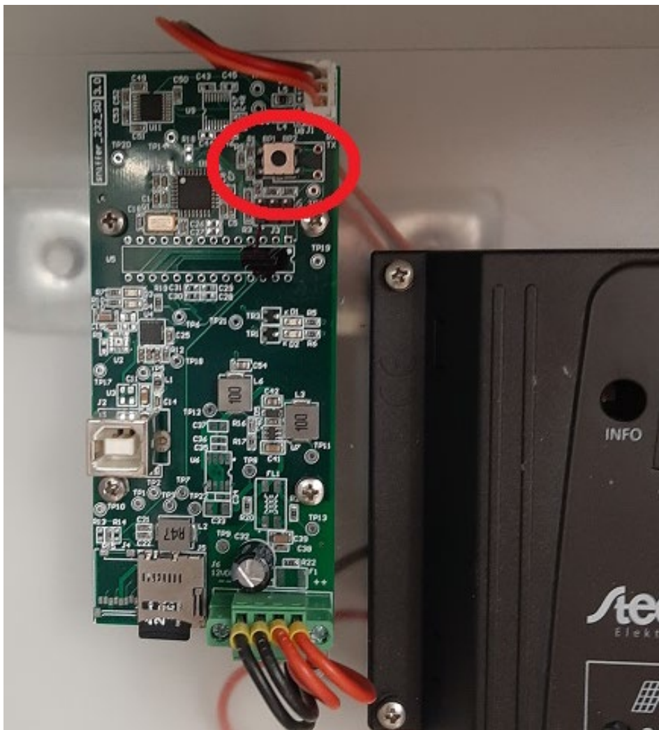
Figure 16: push button to stop the recording on the SD card
