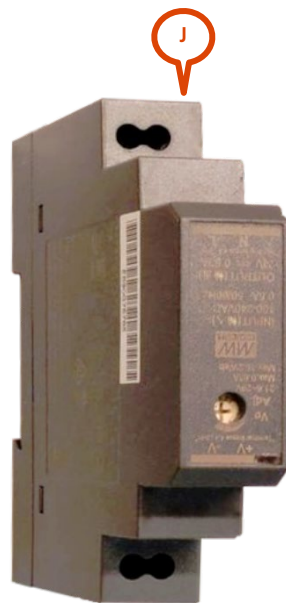
Figure 23: optional transformer for the relay board
