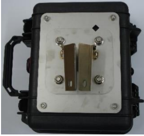
Figure 3: 45° oriented conical bracket
