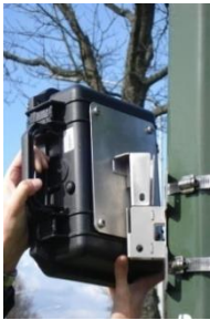
Figure 8: pole bracket + rear bracket
