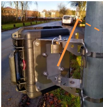
Figure 22: clamping screw with TMS-SA at a different angle
