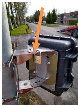
Figure 21: orientation at -45° with clamping screw and optional padlock
