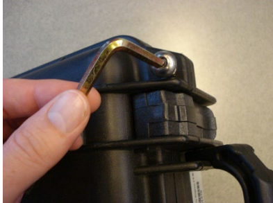
Figure 28: security tool - opening the housing
