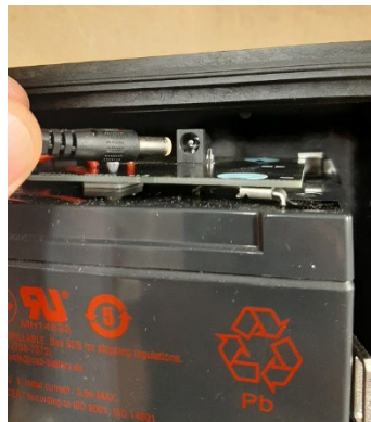
Figure 29: DC plug - charging the battery
