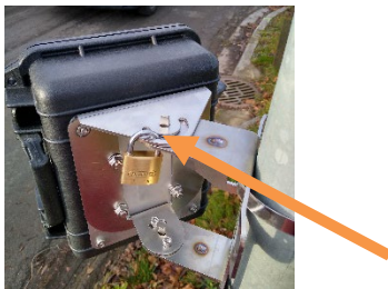
Figure 23: insertion space for anti-theft padlock
