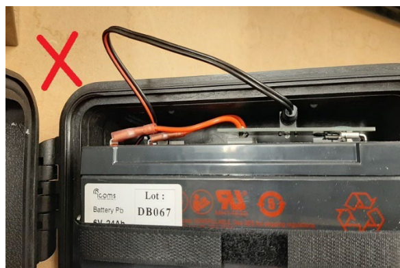
Figure 30: wire to secure above the battery
